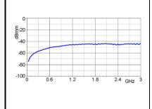
**RF-E 05** With this probe you are able to register selectively electrical fields on layouts and component area of flat units. The breadth of the field electrode is about 1 mm. Therefore you can locate electrical fields very accurately. These electrical fields are caused by clocked lines, IC pins and small components.
