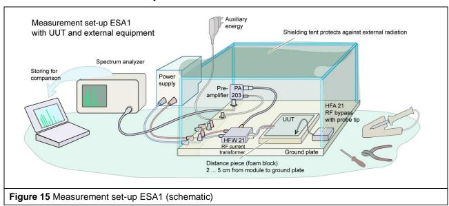
First place the GP 23 ground plate with its socket connectors pointing to the left (under normal conditions) and set up the shielding tent (description in section 2.2).
