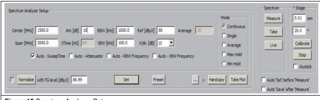
Figure 19 Spectrum Analyzer Setup
