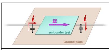
You can also establish a capacitive connection from GND or Vcc, for example, to the ground plate.
