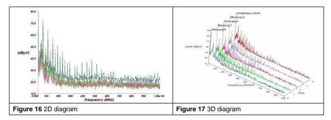
It does not matter if the measured data was recorded in different frequency ranges. Individual measurement curves can be displayed or hidden and each curve can be assigned a certain color or description to provide a better overview. Furthermore, gridlines allow the developer to compare measurement curves very precisely in the linear or logarithmic 2D diagram.
