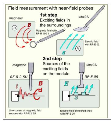
Begin by determining the magnetic and electric fields in the vicinity of the modules. These fields incite the whole metal system of the unit under test to oscillate (exciting fields) and must finally be reduced. You should use near-field probes with a bigger probe head, i.e. the probe RF-R 400-1 for magnetic and the probe RF-E 02 for electric fields.
