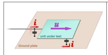
The distance between the unit under test and the ground plate influences the magnitude of the RF current:
