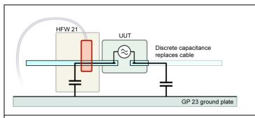
Replacing cables that are not crucial for operation with a link to the ground plate:
