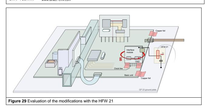
Tap the voltage directly at the GND terminal of the interface plug via a short measuring cable to the COM port of the HFW 21. Thus the modifications that have been made directly on the interface module can be evaluated.
