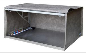
If the tent is set up as shown in **Figure 7**, you can see two press buttons at the upper front edge of the shielding material. Secure these around the front transverse bar.
