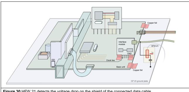
Figure 30 HFW 21 detects the voltage drop on the shield of the connected data cable
